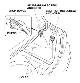
26. Repeat step 25 to install two self-tapping screws/ anchors B on the left side of the vehicle.
